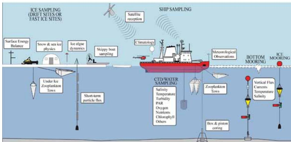
Fig. 2.2-17. Schematic of the scientific equipment used on the Amundsen and at ice camps nearby. (Image: David Barber)
